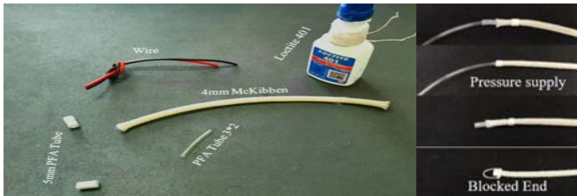
Fig. 2: Fabrication of 4mm McKibben muscles
