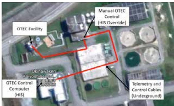
Figure 5.4: Overall layout of OTEC control system
